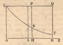
The space described in the time A H with the first velocity continued uniform : space described in the resisting medium, in the same time : : A H P L : area A L S H : : rect. A L  $\times$  P L : rect. A L  $\times$  P S\* : : P L : P S (if A L = subtan. of the curve).
